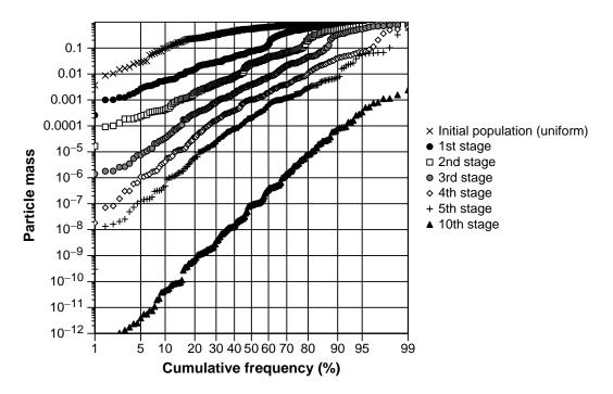
**Figure B-1.** Sequence of asymmetric binary breakages of particles, beginning with a uniformly distributed population, with mass distribution between 0 and 1. Distributions represent particle masses. The mass of the smaller member of a severed pair has the uniform distribution (0, 0.125). The tendency toward linearity at the  $10^{th}$  stage is suggestive of the effect of the Central Limit Theorem.
