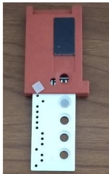
Figure 4. Example of the shape of the TLD-100 dosimeter, also showing the position inside the coded card.
