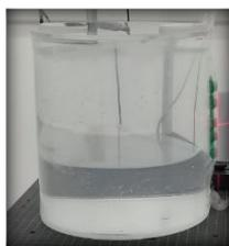
Figure 5. Locally manufactured cylindrical phantom. The cylinder is filled with water for irradiations
