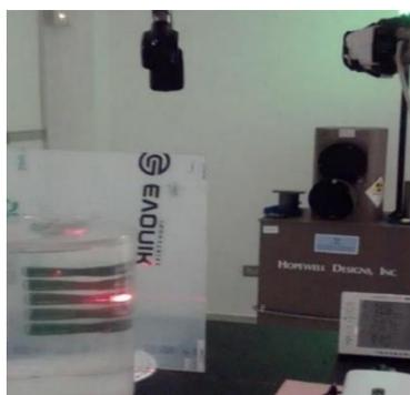
Figure 6. Dosimeter irradiation setup with the  $^{137}\text{Cs}$  reference source on the LAF-RAM LCD.
