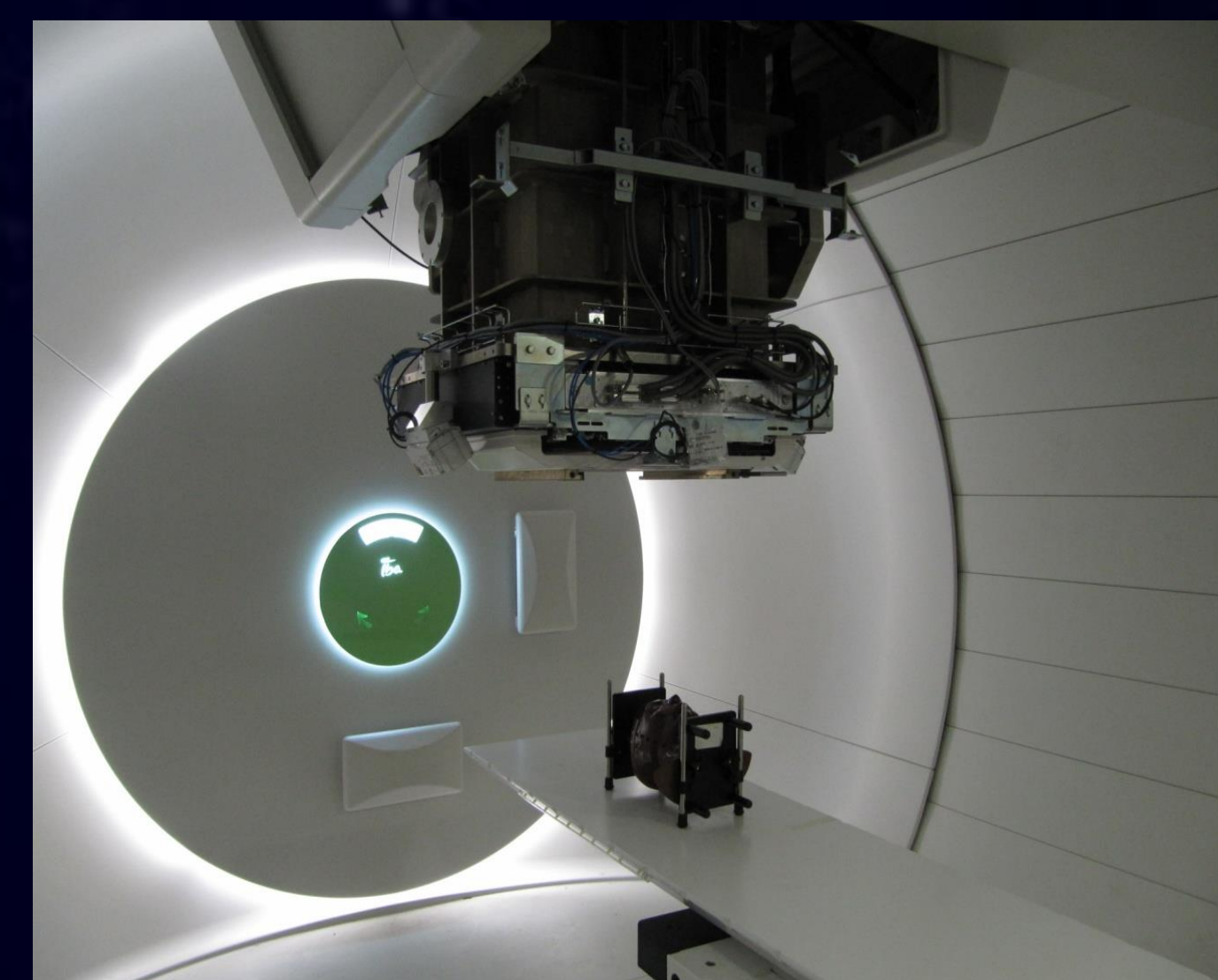
Figure 3 The proton irradiation set up at the pencil beam gantry of the WPE medical cyclotron showing an anthropomorphic head phantom for holding the Extravehicular Visor Assembly (EVVA).
