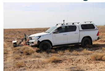
Figure 5: Detection of U-238, Th-232 and K-40 using a gamma ray radiometer (Radiation Solutions Inc., Mississauga, Ontario, Canada) with a 4.2 L thallium-activated sodium iodide detector crystal coupled with a real-time kinematic global positioning system.
