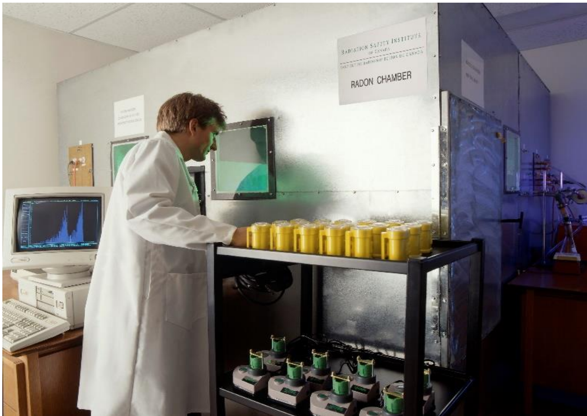
PAD performance testing in the Institute's National Radon Chamber
