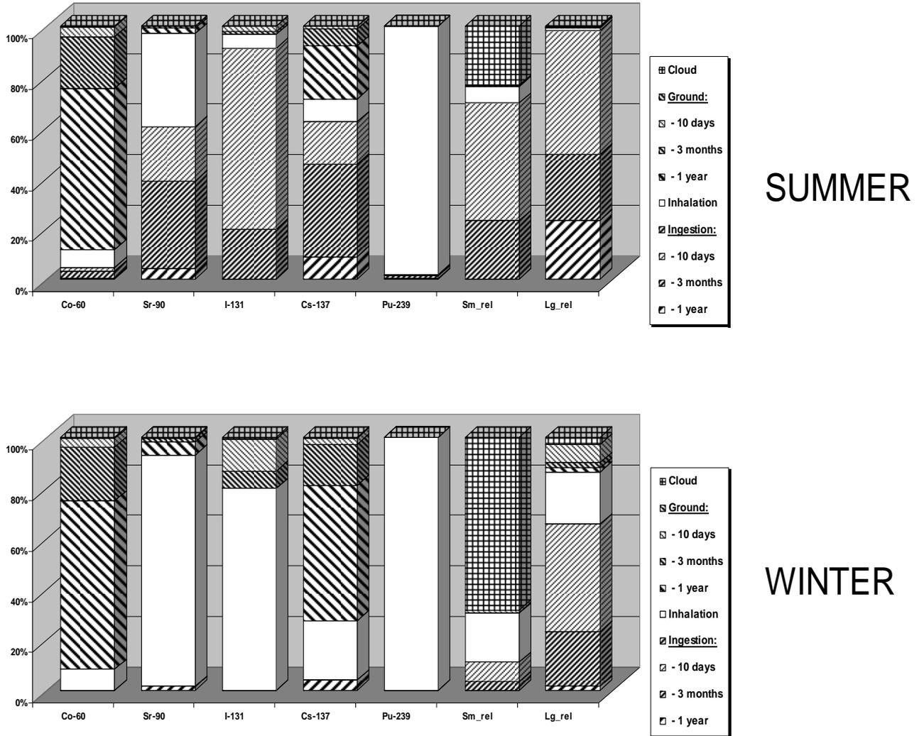
Fig. 4: Examples for the relative contribution of different pathways to the total dose
