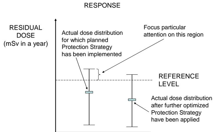
Fig. 3b: Actual dose distribution after implementing the planned protection strategy (left) and optimization (right)
