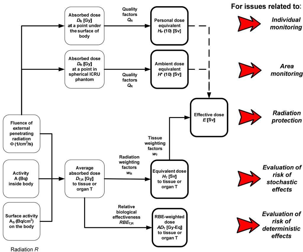
Figure 2: Basic dosimetric quantities and their application.
