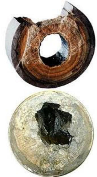
Examples of Heavy Scaling within Oil Production Pipelines (Statoil)
