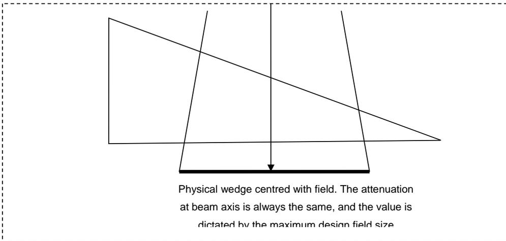
Physical wedge centred with field. The attenuation at beam axis is always the same, and the value is dictated by the maximum design field size
