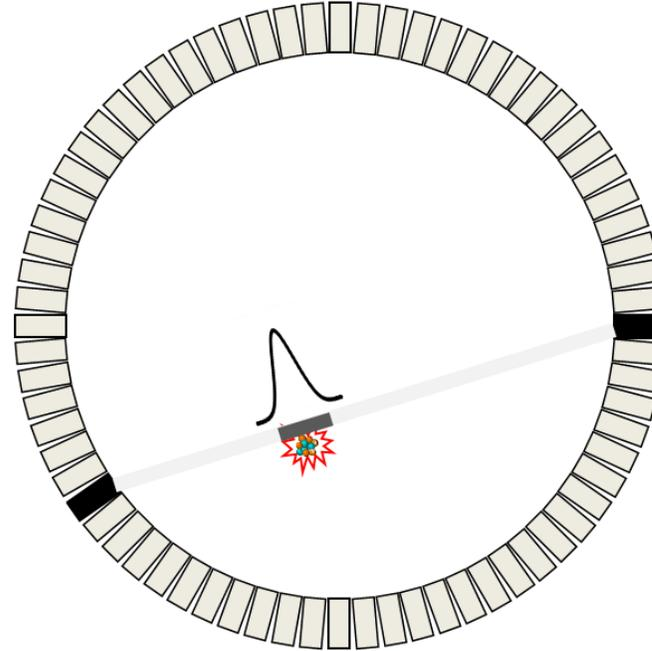
In TOF, a position is calculated along the LOR, and the probability of the event is assigned only to a small segment of the LOR
