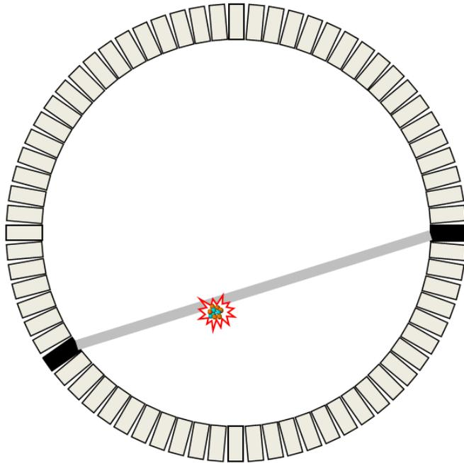
A detection within the coincidence timing window is assigned to the LOR, with uniform probability
