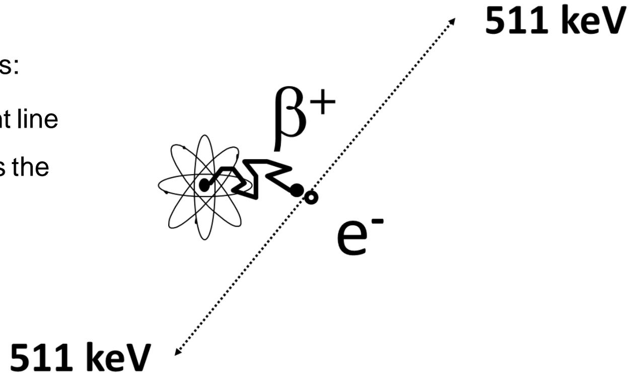
Fig. 2.1. The annihilation of the positron with its anti-particle, an electron, results in the emission of two photons of 511 keV each, almost on a straight line.
