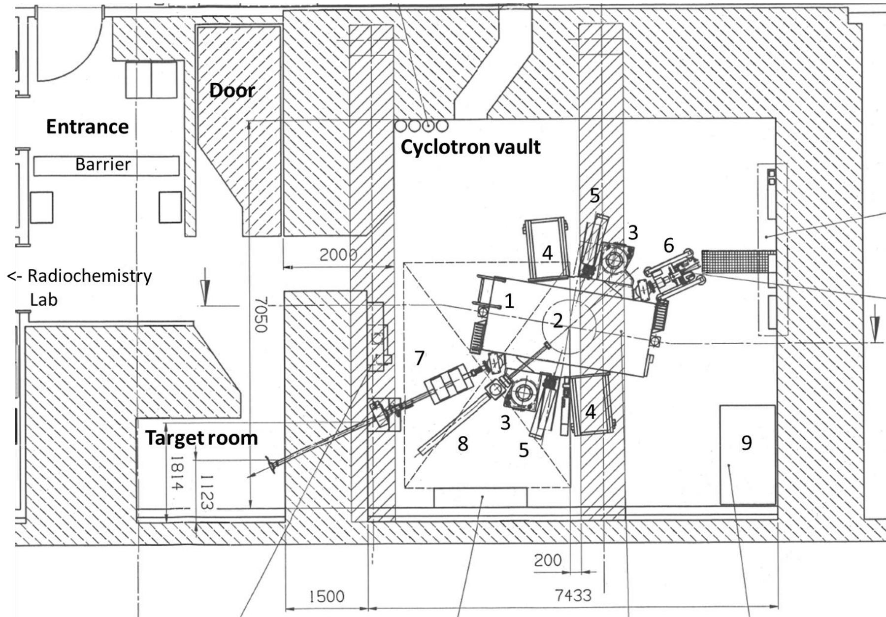
Example of a cyclotron vault and surroundings for an "unshielded" 32 MeV device (installed 1991)
