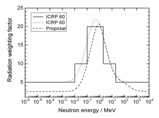
Figure 2. Radiation weighting factor,  $w_R$ , for neutrons versus neutron energy. Step function and continuous function given in Publication 60 (ICRP 1991) and function proposed in this report.
