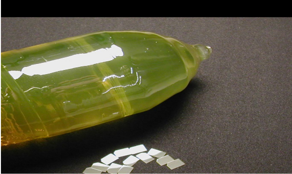
Fig. 1. Al 2 O 3 :C-Mg crystal and 4 × 6 × 0.5 mm 3 FNTD (Akselrod et al., 2003).
