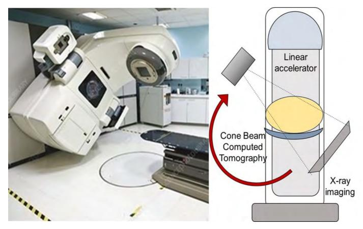
Fig 2. Cone beam CT imaging system on a linear accelerator
