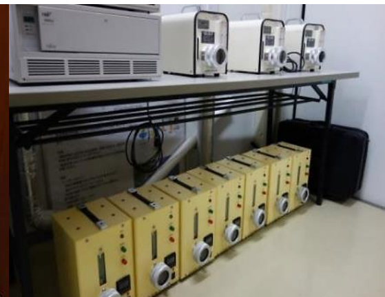
Air sampler for dust and iodine
