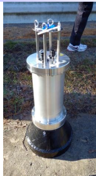
J-sub D: Water proof LaBr3 spectrometer with skirt shape detection window
